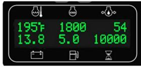
The Vehicle Monitor will display the J1939 Code and a code description for the Operator and/or Technician to use evaluate engine problems. If only a numerical fault code is given, see Diagnostic Trouble Codes (DTC) listing.
